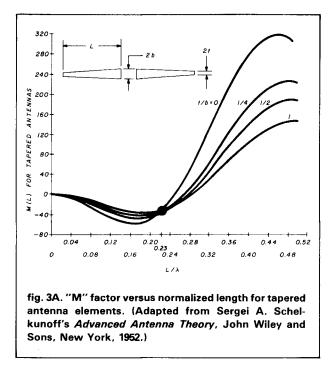
line used for matching two different impedances (see **fig. 1**). Notice that each section of the exponential transmission line has its own surge or characteristic impedance. An impedance transformation occurs in either direction as a result of the taper. Consequently a tapered antenna element can be considered as a tapered exponential transmission line that has an average characteristic impedance described as a geometrical mean of its diameter.
